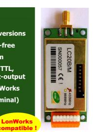
The LC20 radio transceiver meet an increasing demand : It enables wireless communication between any serial devices without any specific study. All the intelligence and knowledge is integrated inside the radio module.
