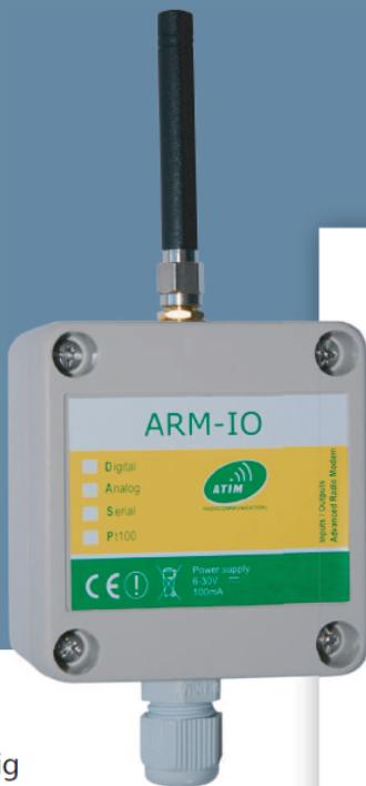
Radio modems ARM-IO 868MHz 25mW have been developed in order to answer to a big need of wireless data transmission in disturbed industrial environment (400m), and in outside environment until 1000m LOS (line of sight).
